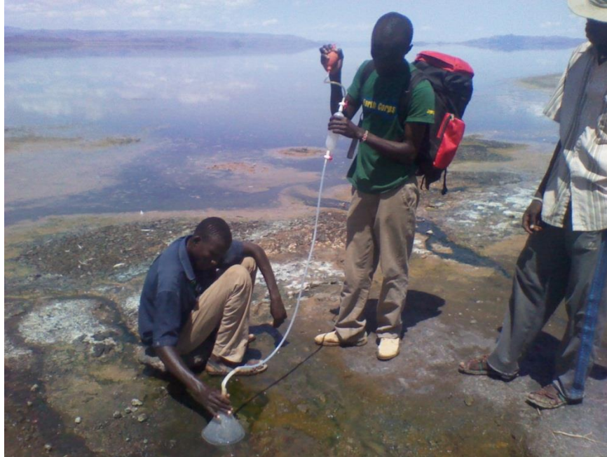
Plate 5: Field water sampling of Lake Logipi hot spring discharge
