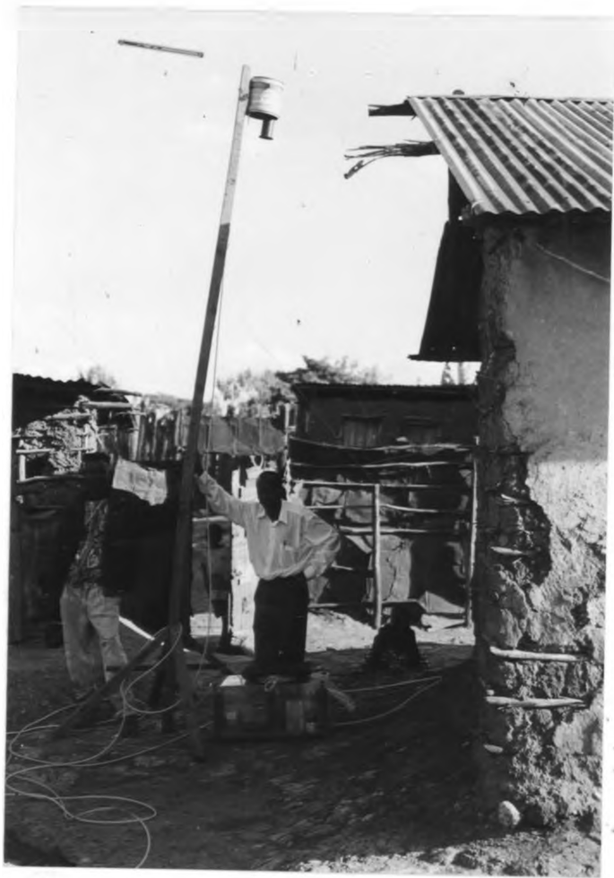
Fig 4.2f: Site E, “Gent” SFU sampler at a height of four (4) metres above the ground.
