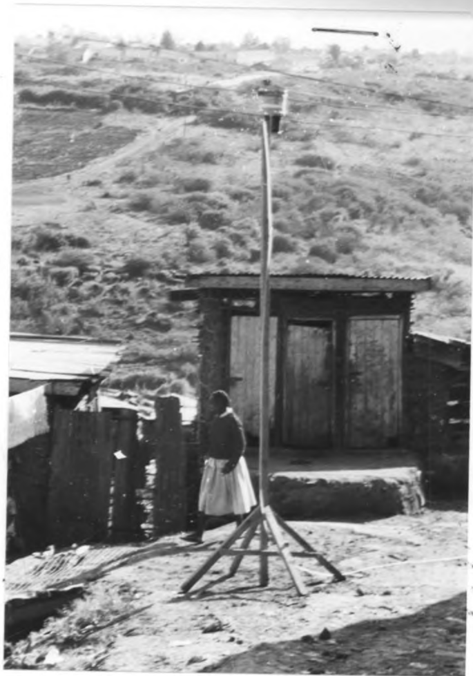
Fig 4.2b: Site A, "Gent" SFU sampler at a height of four (4) metres above the ground
