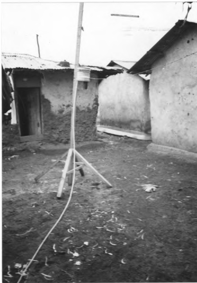
Fig 4.2c: Site B, "Gent" SFU sampler at a height of two (2) metres above the ground .
