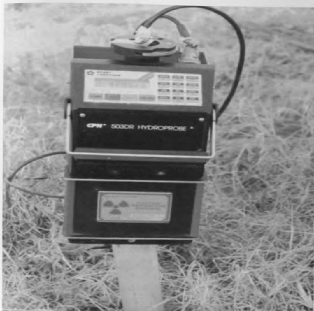
Plate 8: The Neutron Probe model used during soil moisture data collection
