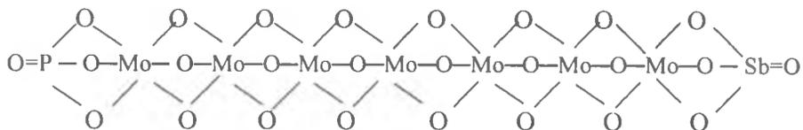
On the other hand, the structure of the final reduced molybdenum blue ( $\text{H}_2\text{PO}_4\text{Mo}_7\text{O}_{12}\text{SbO}_4$ ), where molybdenum has coordination number and oxidation number of 4, may be illustrated as follows:
