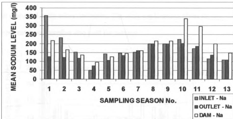
Figure 19. Variation of Sodium Concentration from Inlet, Outlet & Nairobi Dam Water with Sampling Seasons.
