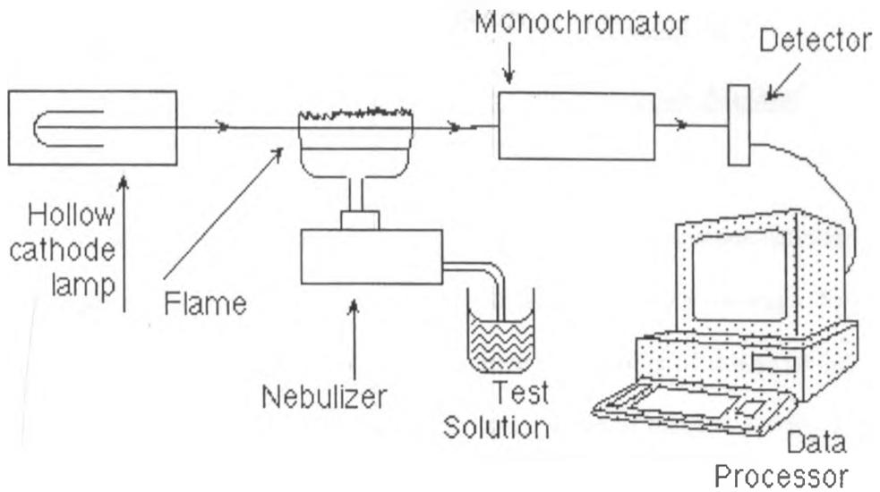
Figure 3. Schematic diagram showing components of an Atomic Absorption Spectrophotometer.
