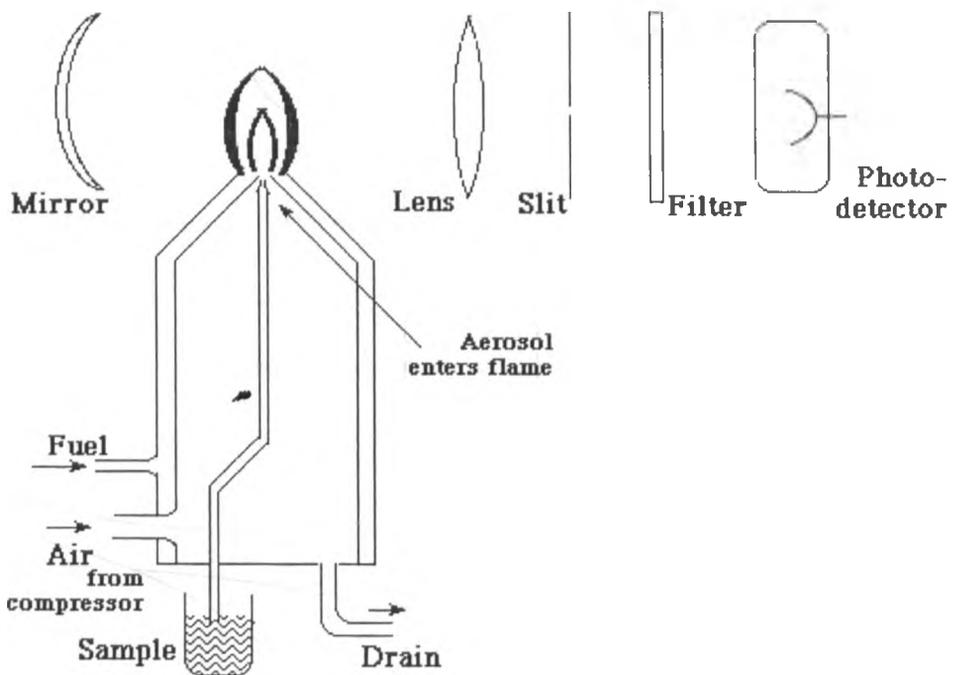
Figure 4. Schematic diagram showing components of a Flame (Emission) Photometer.
