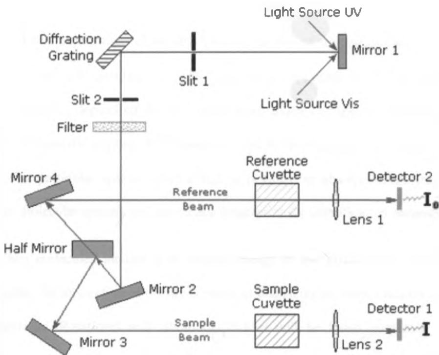
Figure 2. **Schematic diagram depicting Instrument modules for measuring UV/Visible Absorption of radiation.**
