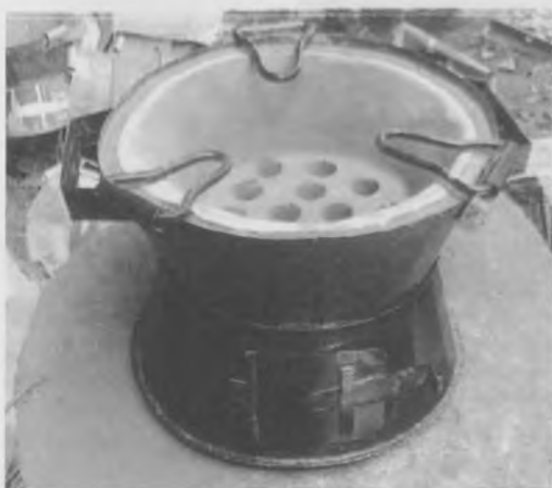
Figure 2- 3: A common energy saving jiko
