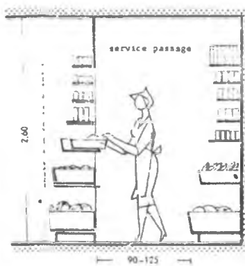
11 Shop wall with service passage at back for replenishing goods. Empty drawers are replaced.
