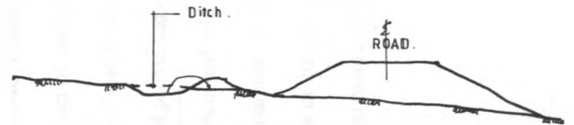
III. cut-off ditch
