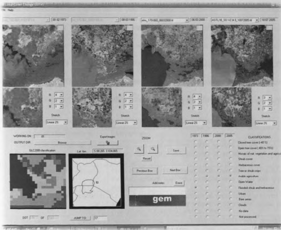
Figure 6: Example screen shot of GUI used to assess wetland land cover change at Kusa Swamp IBA around Lake Victoria. The four boxes cover, from right to left, the different time periods used in the study and show a decline in flooded vegetation
