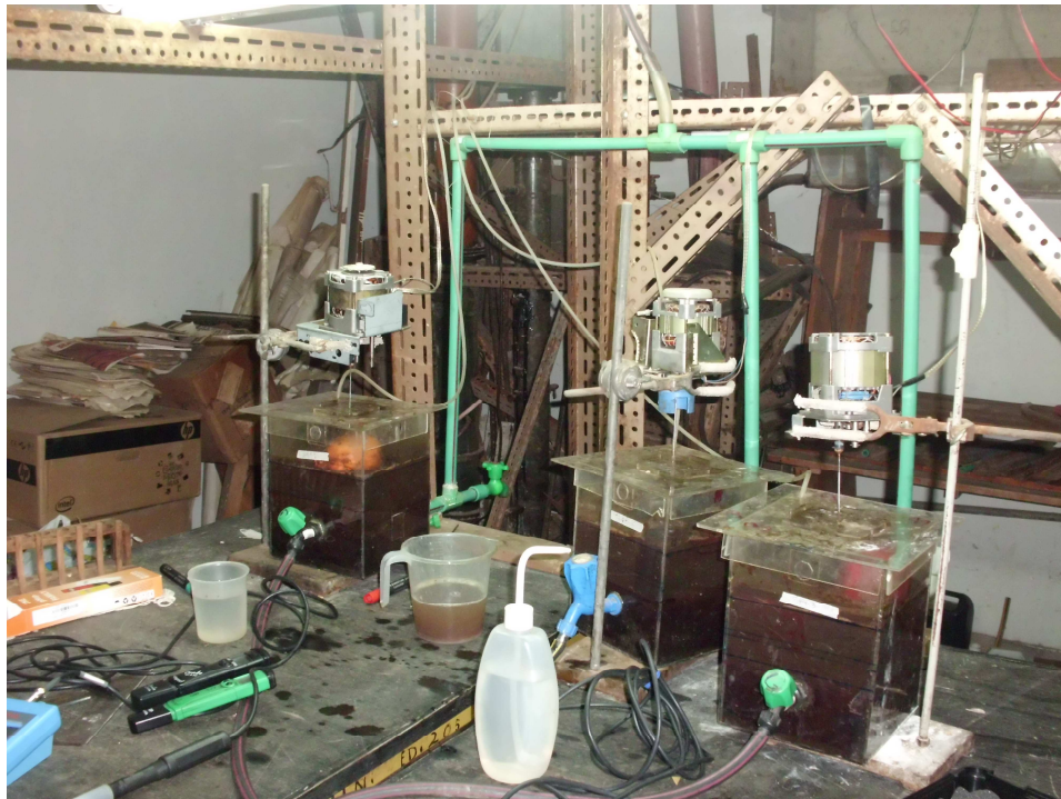
Figure 3.2: Perspex-glass SBR Vessel (adapted from Norcross, 1998)
