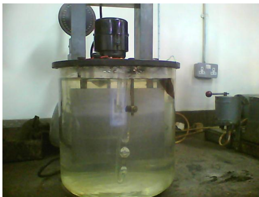
Figure 3.13: Set up for determination of kinematic viscosity
