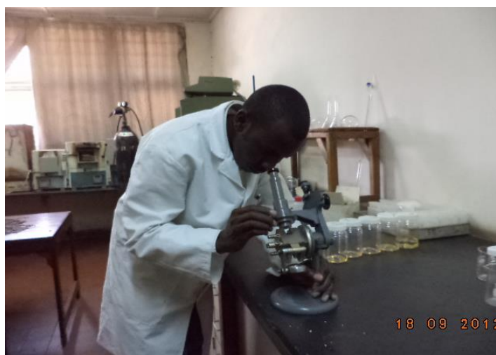
Figure 3.14: Determining the refractive index using an Abbe refractometer.
