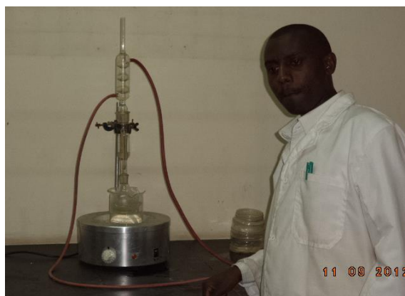
Figure 3.12: Extraction of castor oil using the soxhlet extractor in a water bath.
