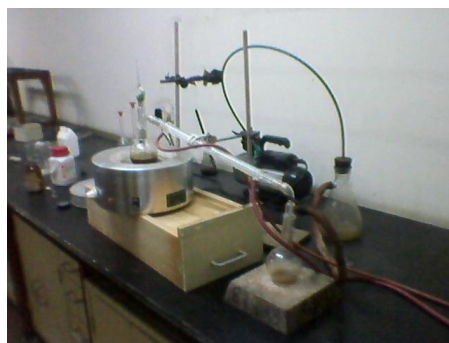
Fig 3.15: Laboratory set up for dehydration of castor oil.
