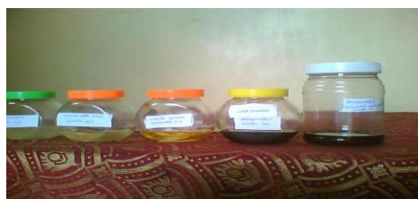
Figure 3.17: Neutralized, crude solvent and cold pressed oil and dehydrated castor oil.
