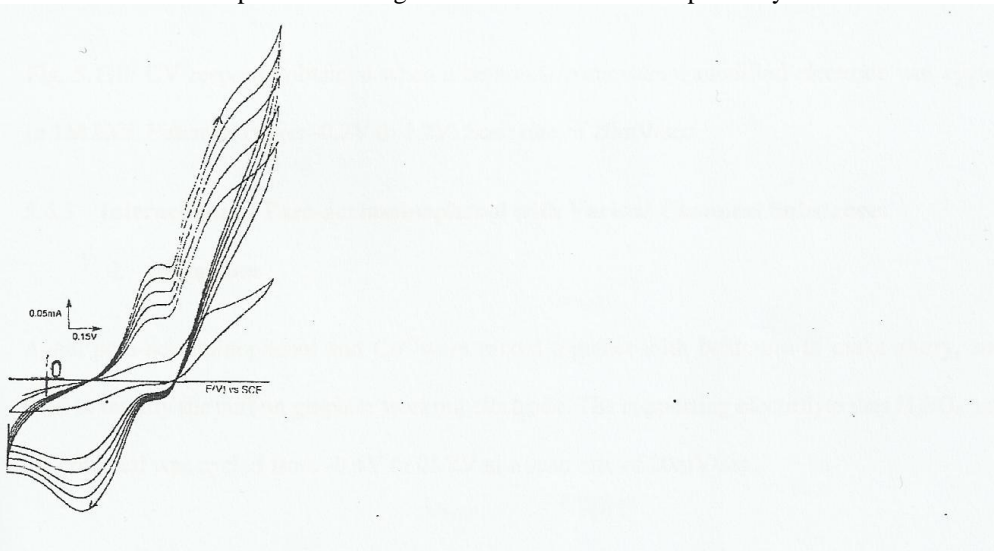
Fig. 5: CV response obtained when a bentonite-paracetamol modified electrode was cycled in 1M H 2 SO 4 . Potential range: -0.4V to 1.2V. Scan rate of 20mV/sec
