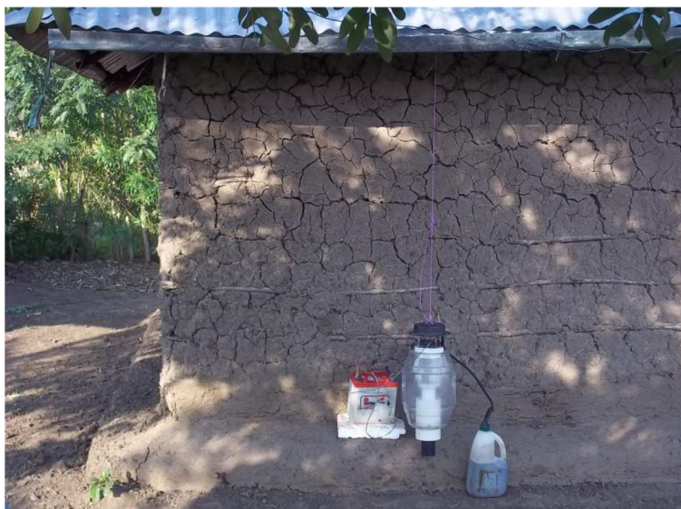
Figure 1 A picture of an outdoor trapping system baited with the Mbita odour blend augmented with carbon dioxide produced by fermentation of 250 g molasses using 17.5 g dry yeast mixed with 2 L water. Carbon dioxide was produced in a plastic container and delivered into the MM-X trap through silicon tubing.
