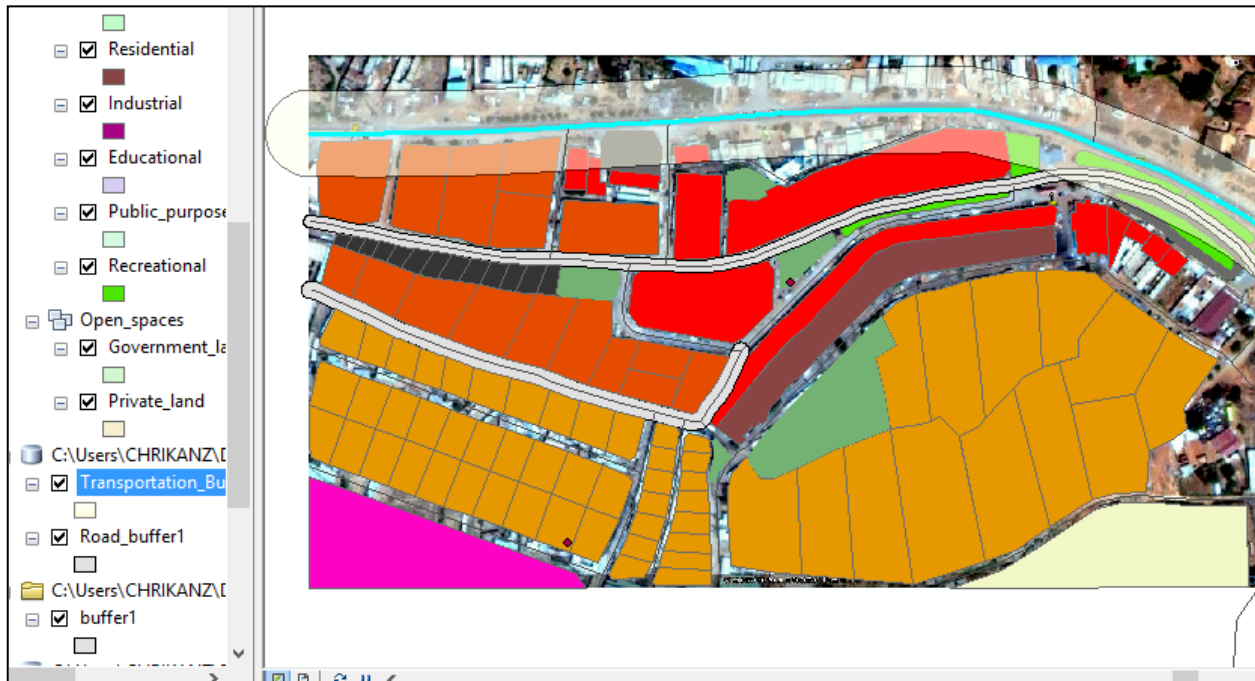
Figure 19: A buffer showing encroachment index on the A3 highway in Mwingi town.
