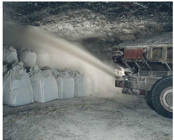
FIG. 6. The remaining space of a chamber is infilled by tailings jettied in
