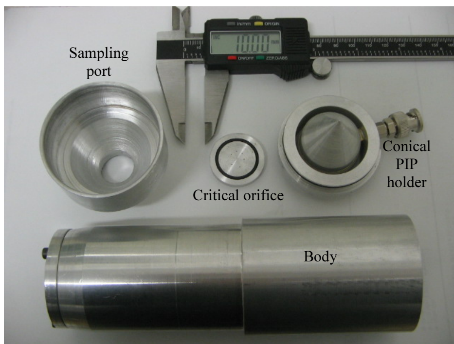
FIG. 2. RPD monitor components investigated for the losses assessment
