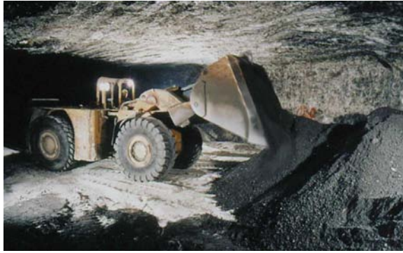
FIG. 1. Dumping of bulk material
