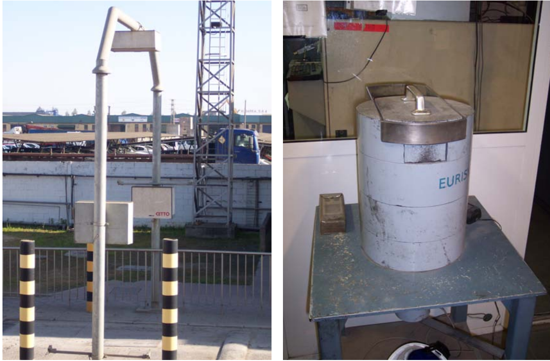
FIG. 1 Radioactivity detectors are distributed in some places of the recycling steel factory.
