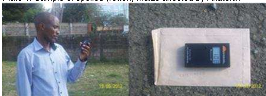
Plate 2: Solar irradiation measurement during the performance of the experiment and the gadget used (Daystar DS-05A Solar Digital Meter)
