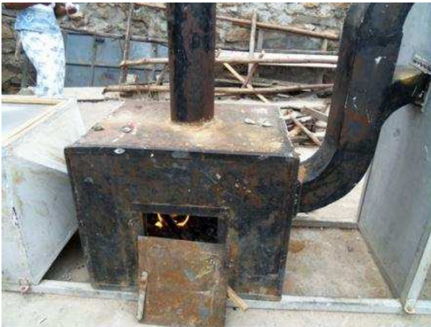
Plate 4: Woodfuel burning in the back-up heater to supplement the solar collector heat during the performance of the experiment
