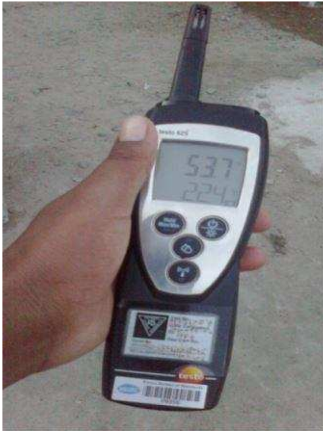
Plate 5: Hygrometer used in determining ambient relative humidity
