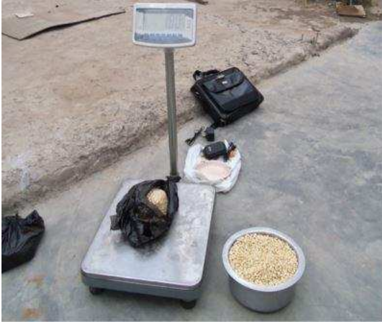
Plate 3: Maize sample preparations; measuring the mass of the grains using weighing balance
