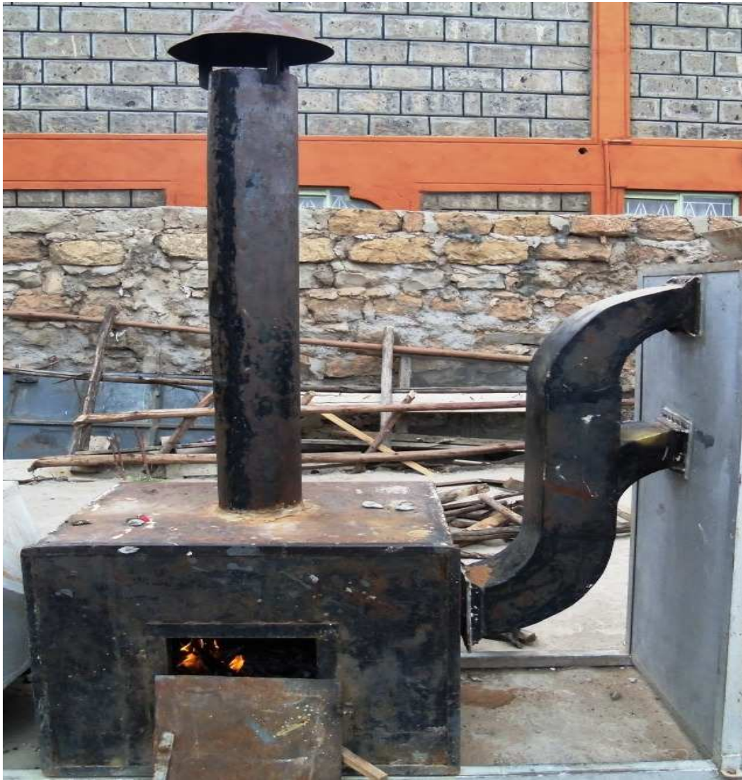
Plate 5.2: Pictorial view of the back-up heater structure of the dryer
