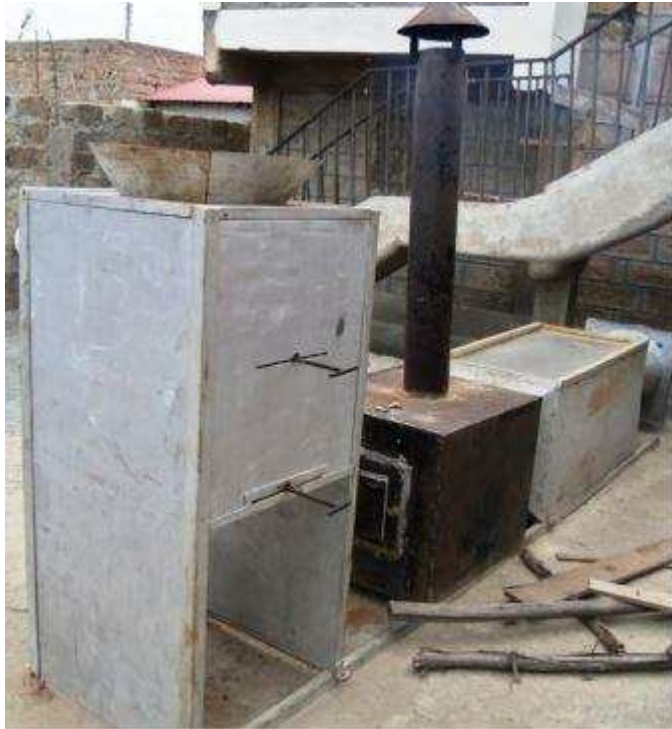
Plate 5.3: Pictorial view of the assembled maize grains dryer.
