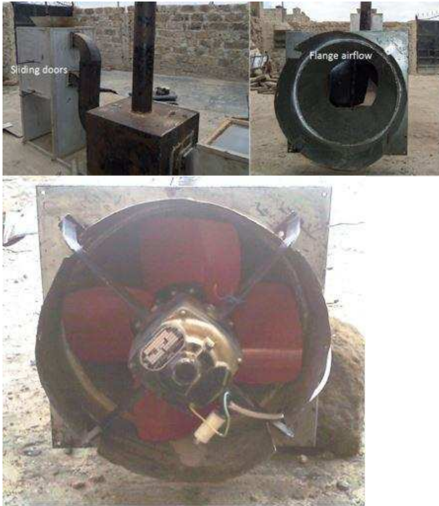
Plate 6: Illustration of (a) sliding doors in the drying chamber, (b) flange air regulator mechanism and (c) installed vane axial fan in the assembled maize drier.
