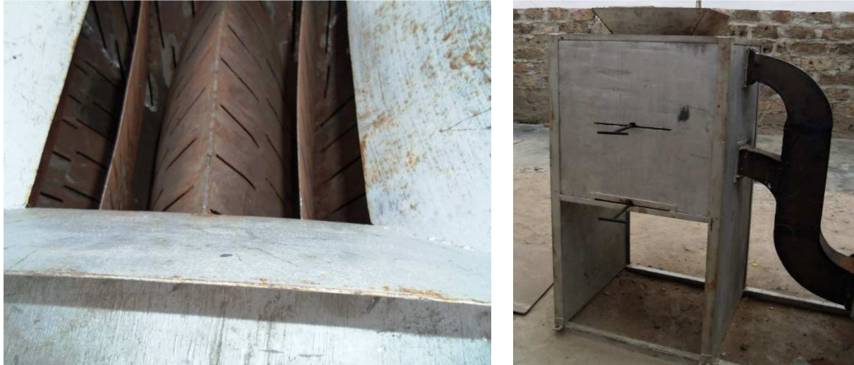
Plate 5.1: Pictorial representations of the drying chamber and trays for the dryer.
