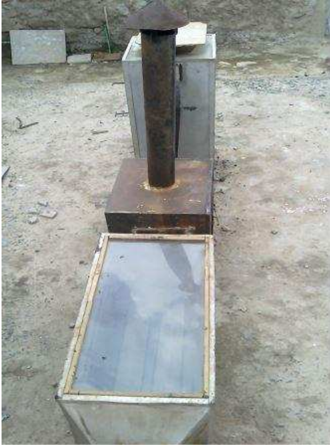
Plate 5. Illustration of plan view of solar assisted maize dryer
