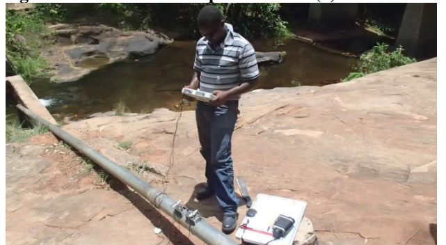
Figure 7-18 Measuring Flow in a Pipe
