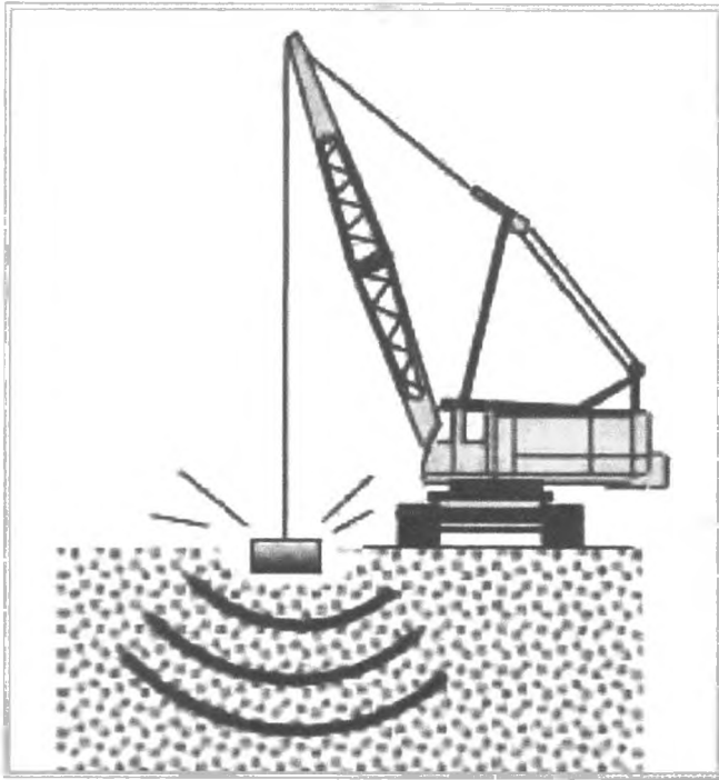
Figure 5.1 Compaction methods to accelerate settlement rates
