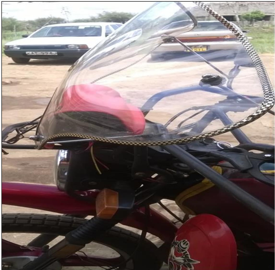
Plate 14: Visors and Side Guard Installed on a Motorcycle
