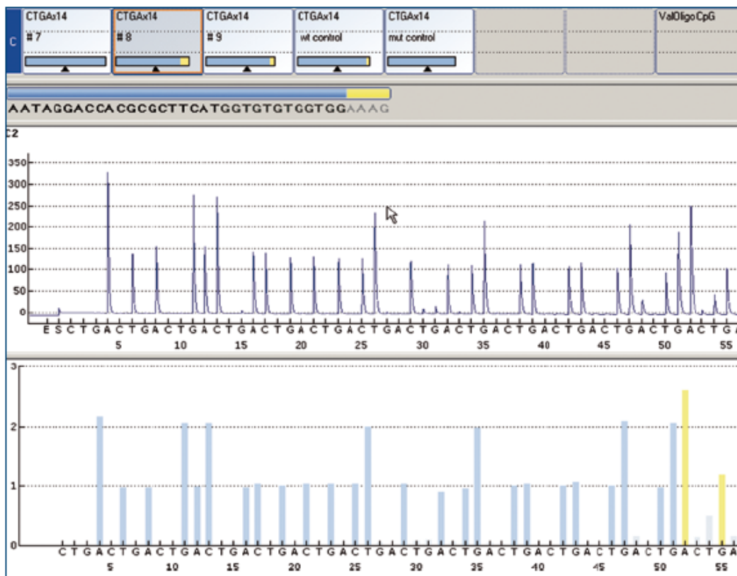
Figure 3.7: Quality Analysis Checks During Sequencing Run; Blue (Passed), Yellow(Check), Red (Failed) (Source: Qiagen technologies)
