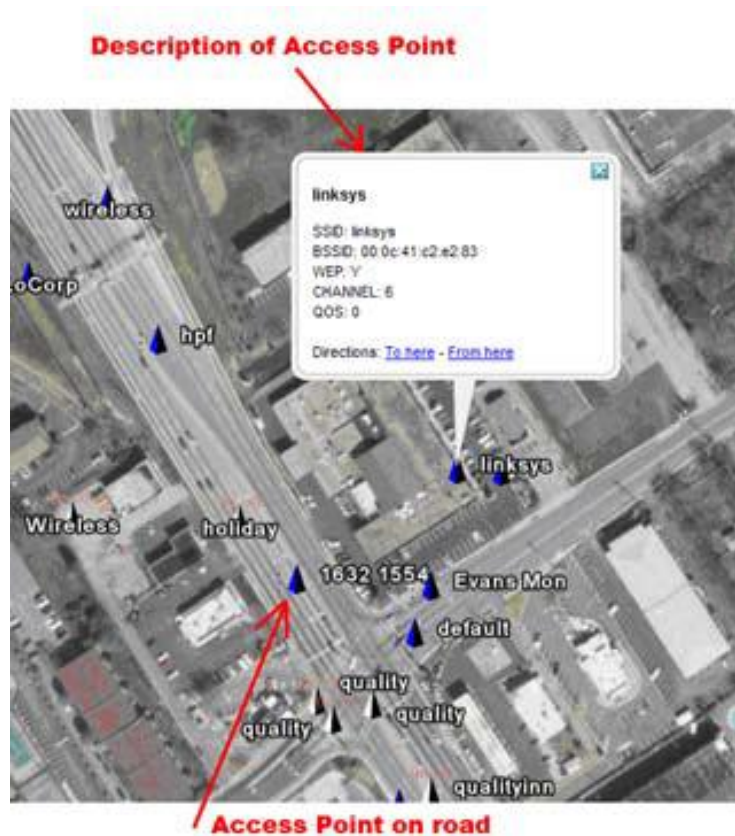
Figure 2.4 WiGLE data showing in Google Earth (Source: Google Earth on 15 th April 2014)
