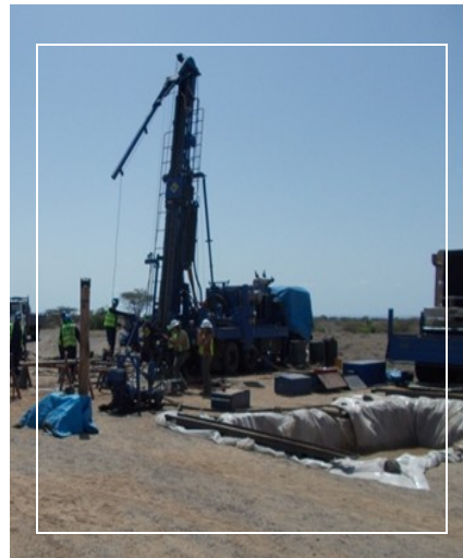
The drilling rig at the West Turkana site. Scientists are extruding a recovered core section of 3m length.
