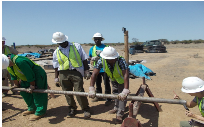
Extrusion of the sediment core from the drill casing: Prof. Andy Cohen (USA), Dr. Craig Feibel (USA), Prof. Daniel Olago (University of Nairobi), Mr. Leslie Dullo (University of Nairobi), Mr. Benson Kyongo (National Museums of Kenya), Dr. Sarah Ivory (USA).
