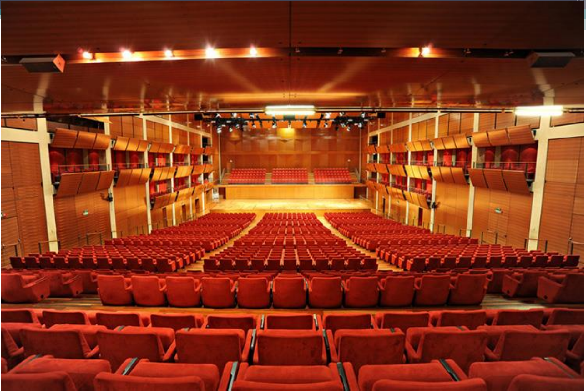
Auditorium del lingotto Torino, Italy. Notice the curved balcony sound reflectors
