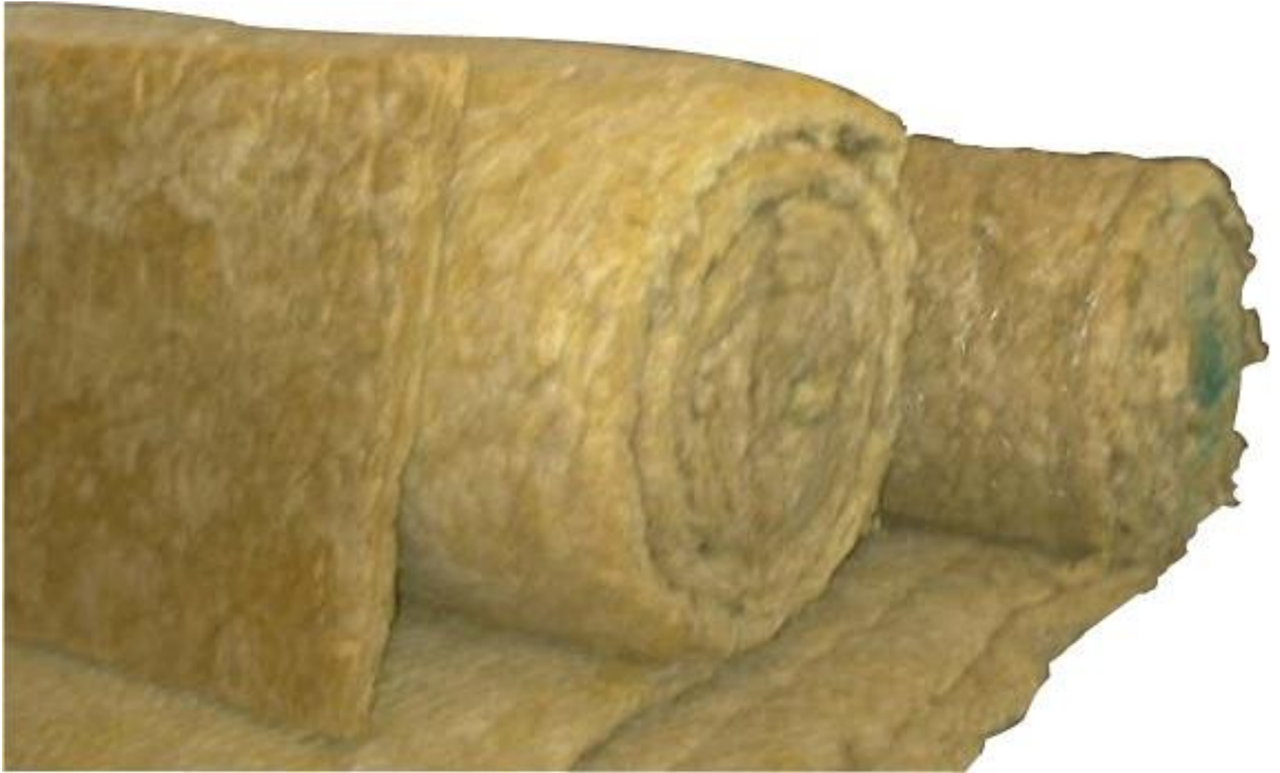
Porous absorbent: Mineral wool
