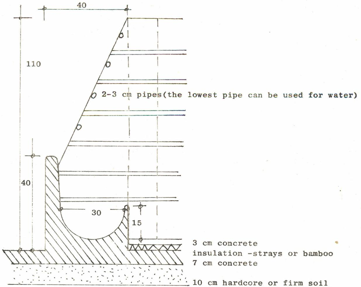
Figure 26. Trough and frontwall of pigpen.
