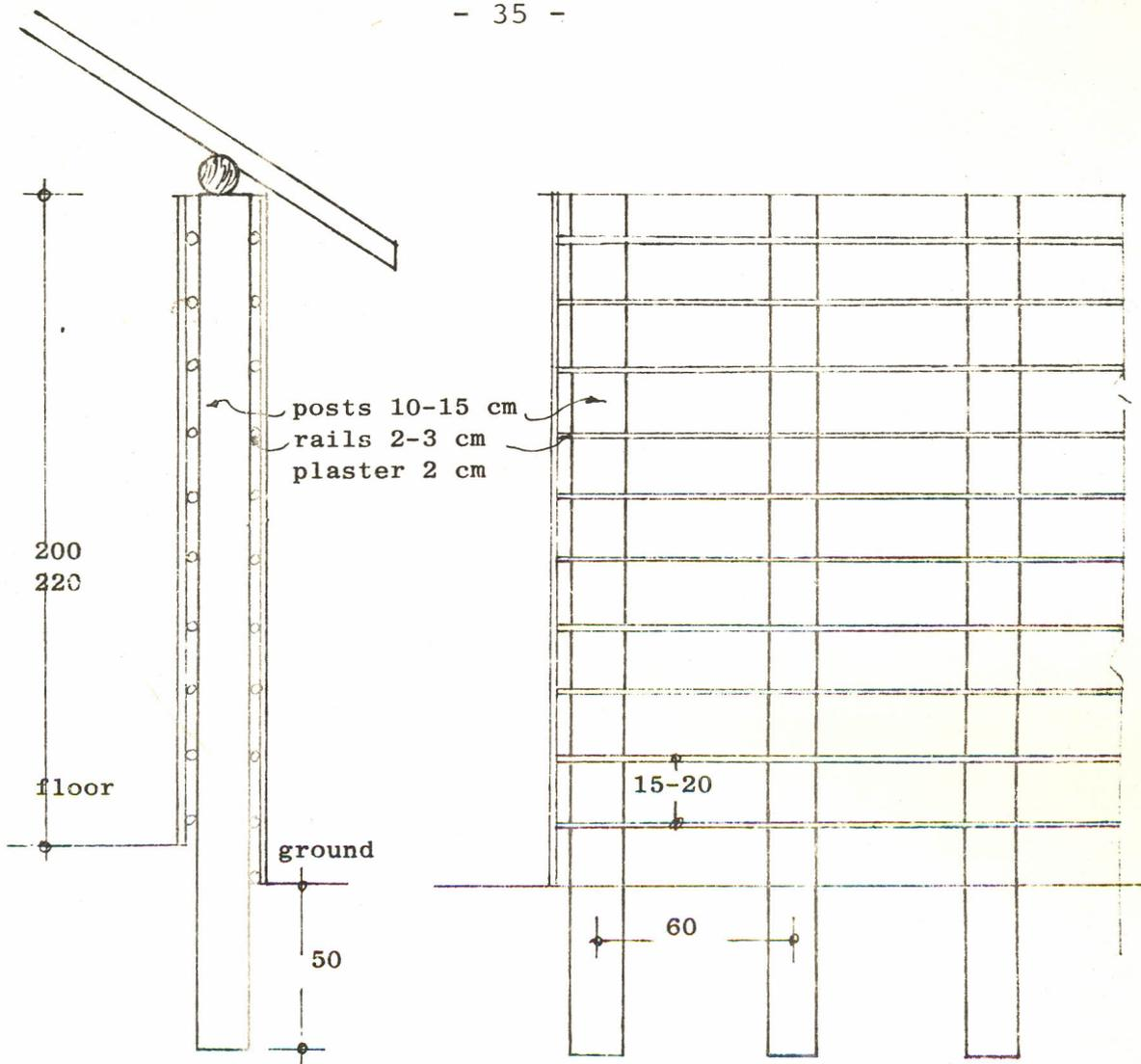
Figure 13 Mudwall-section and side view
