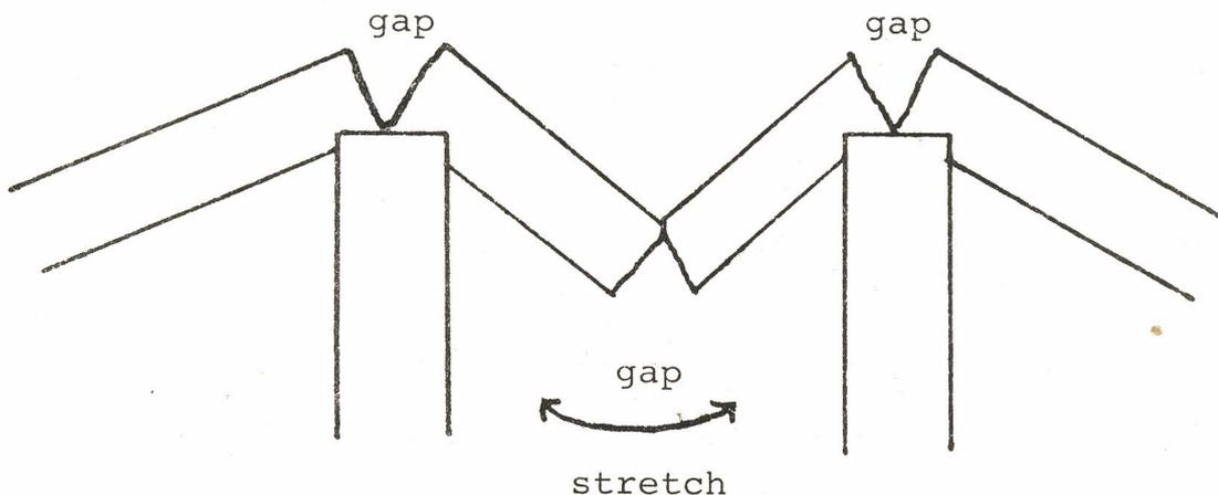
Side view - without reinforcements gaps occur on the stretching side.
