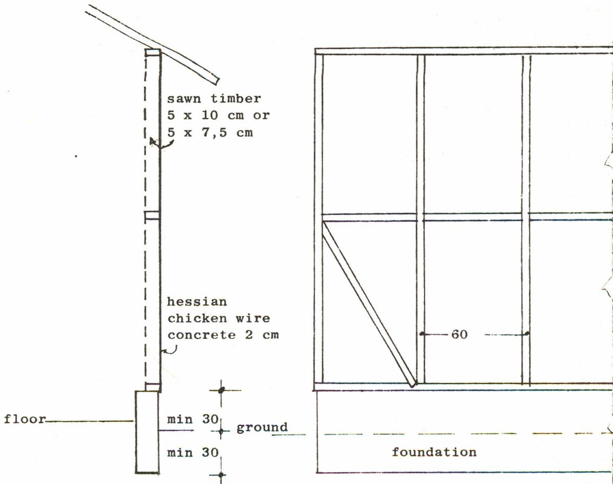
Figure 15. Hessia - concrete wall-section and side view
