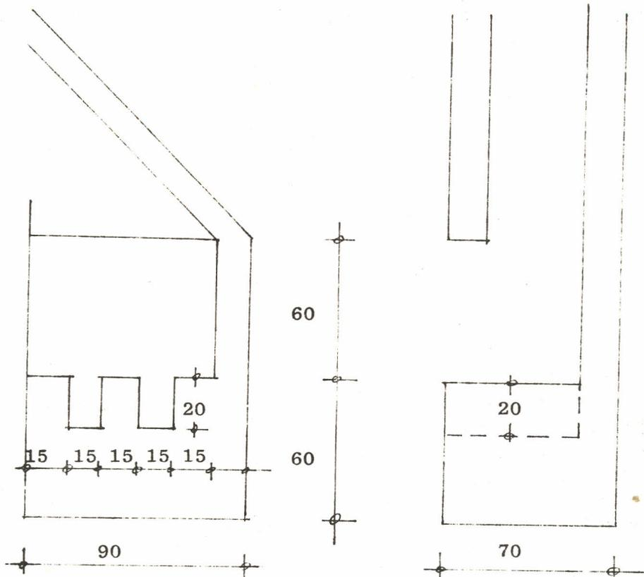
Figure 31. Cooking place-front view and section
