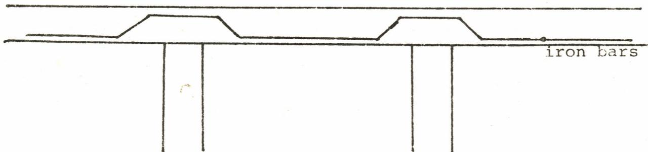
Side view - with reinforcement. The iron bars are bent so they lay in the stretching zone of the concrete.
