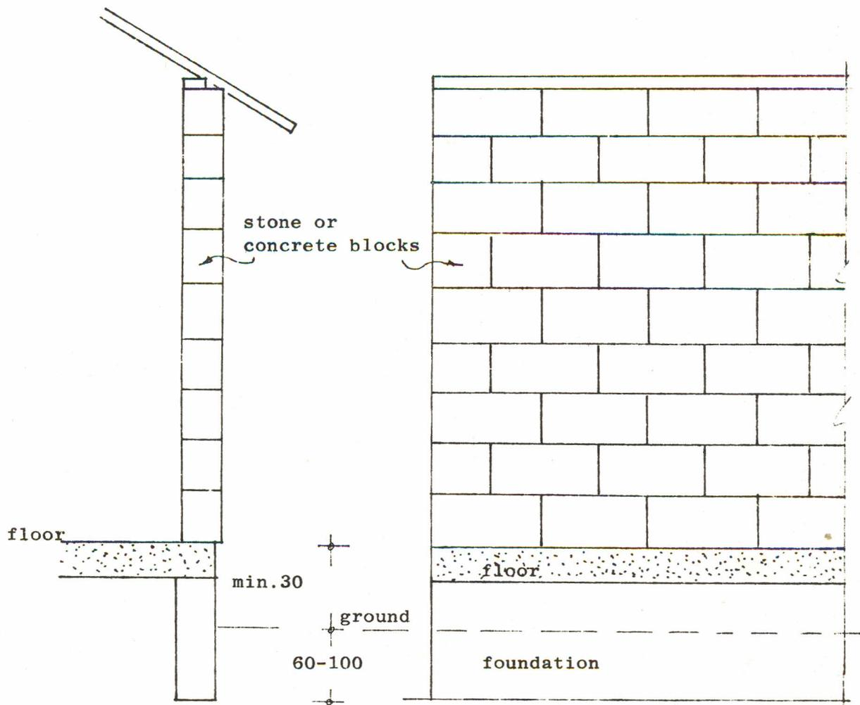
Figure 16. Block wall- section and side view
