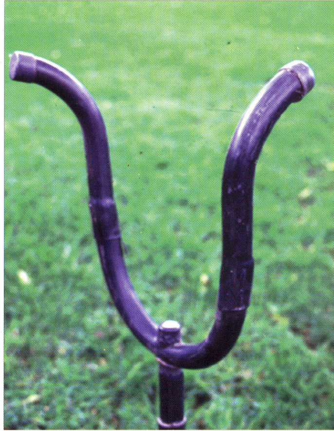
PHOTO 12: JUA KALI REACTION SPRINKLER (UNKNOWN ARTISAN, KANGEITA)
