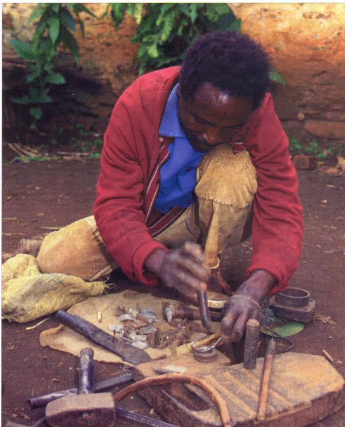
PHOTO 51: ANGELO KATHIA (MERU) WITH THE INSTRUMENTS HIS USES TO MANUFACTURE HIS SPRINKLERS
