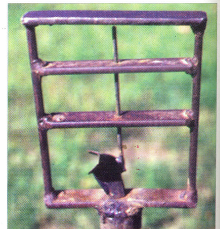
PHOTOS 38 & 39: BUTTERFLY SPRINKLERS, METAL MODELS WITH FIXED SQUARE FRAMES
