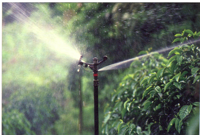
PHOTO 21: IMPACT SPRINKLERS TEND TO PRODUCE BIGGER DROPLETS
