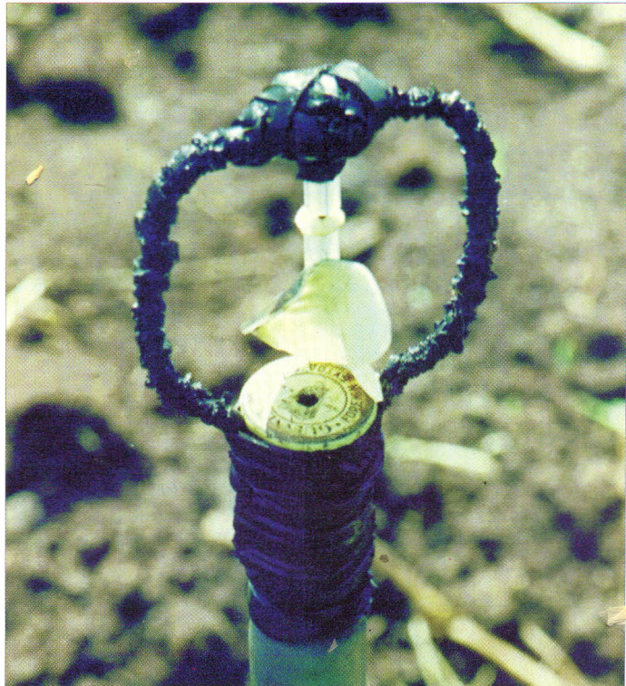
PHOTO 49: PLASTIC BUTTERFLY SPRINKLER MADE WITH SCRAP MATERIALS
