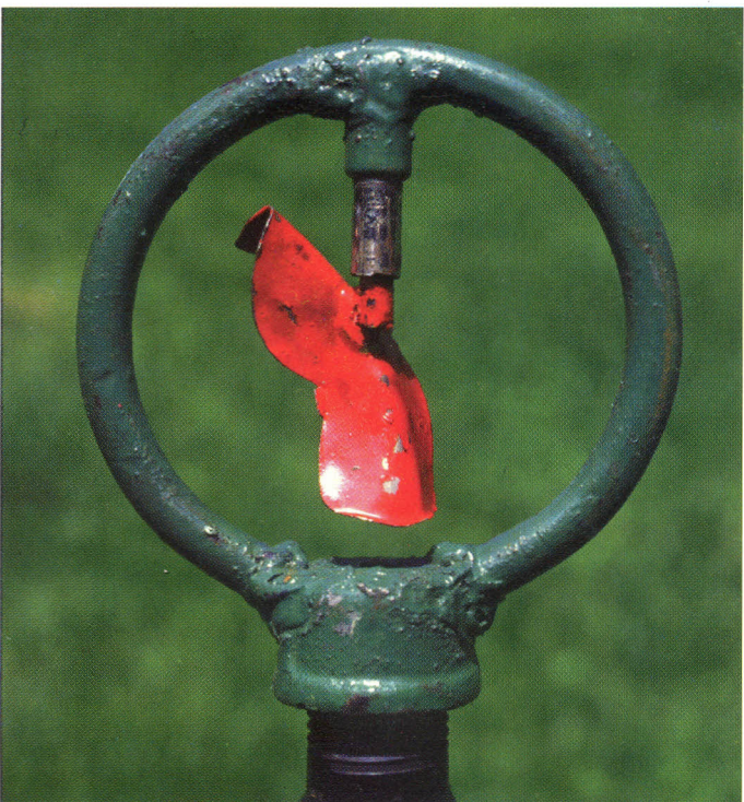
PHOTO 9: BUTTERFLY METAL MODEL WITH FIXED FRAME (KAMAU, EMBU).
