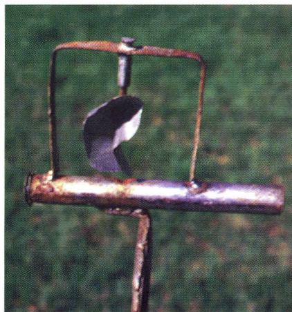
PHOTOS 38 & 39: BUTTERFLY SPRINKLERS, METAL MODELS WITH FIXED SQUARE FRAMES
