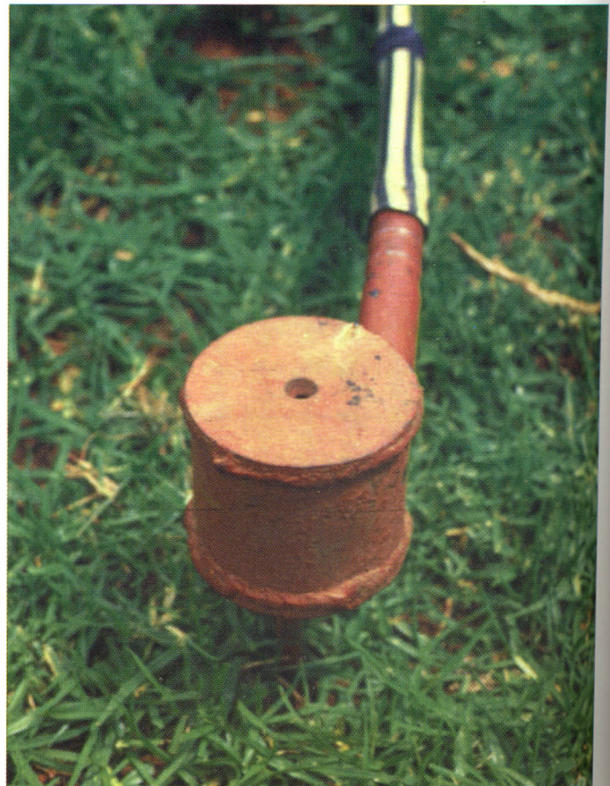
PHOTO 17: JUA KALI STATIC SPRINKLER (SOSPETER KABUA, NAIROBI)
