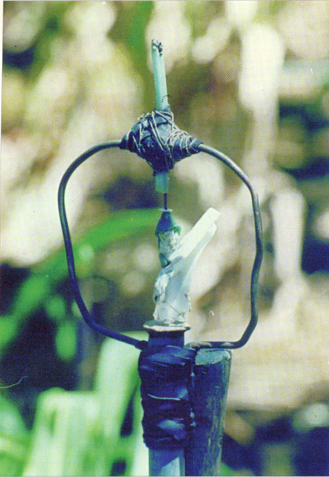
PHOTO 47: PLASTIC BUTTERFLY SPRINKLER MADE WITH SCRAP MATERIALS
