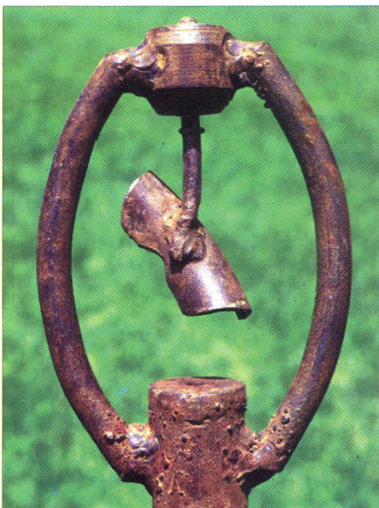
PHOTO 37: CIRCULAR FRAME SPRINKLER
