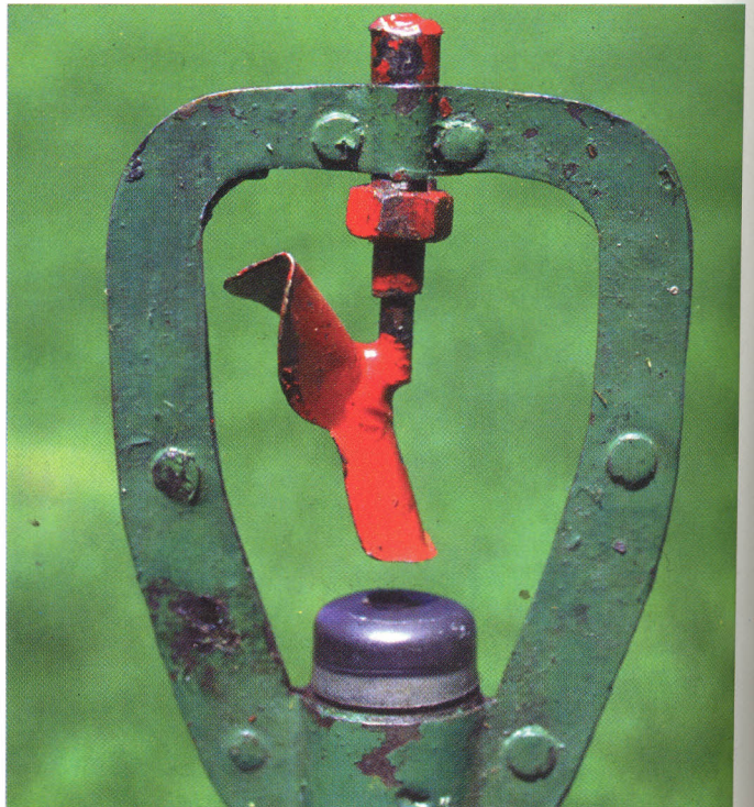
PHOTO 10: BUTTERFLY METAL MODEL WITH ROTATING FRAME (KAMAU, EMBU).
