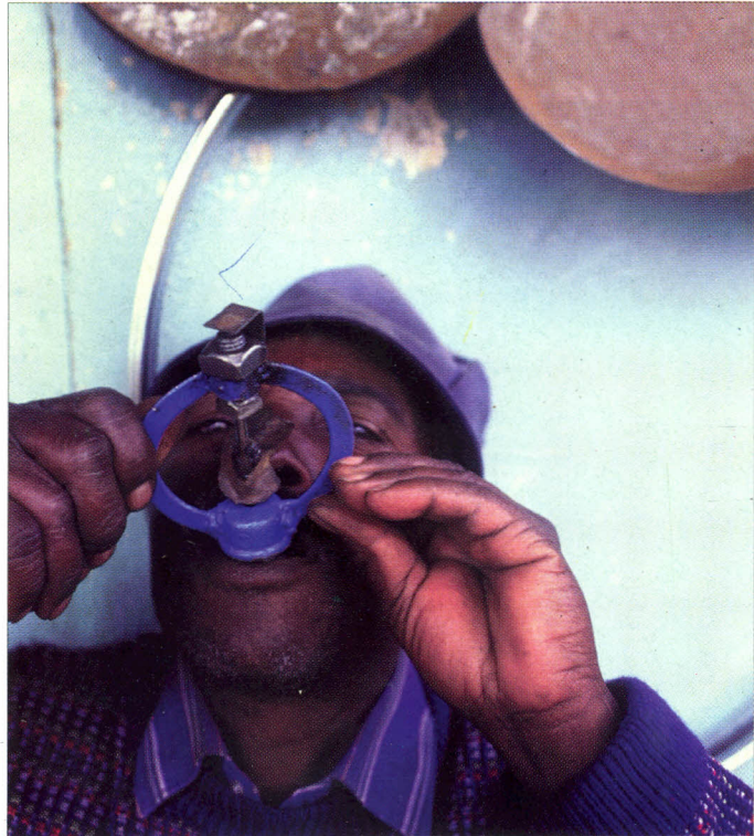
PHOTO 46: TESTING THE NEW SPRINKLER
