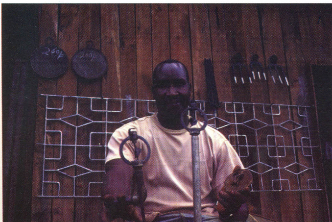
PHOTO 42: PATRICK M'BIJUE MBUI (MERU) AND HIS MODEL OF METAL BUTTERFLY SPRINKLER WITH FIXED FRAME. IN HIS RIGHT HAND IS THE DEVICE HE USES TO BEND THE BUTTERFLY.
