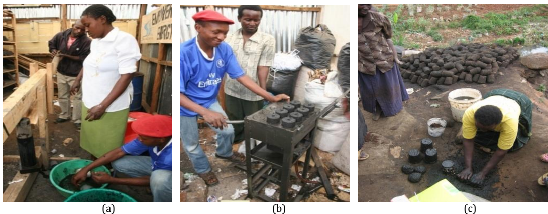
Fig. 1 (a) Wooden manual, (b) Metal manual press, (c) Molding in recycled plastic container containers
