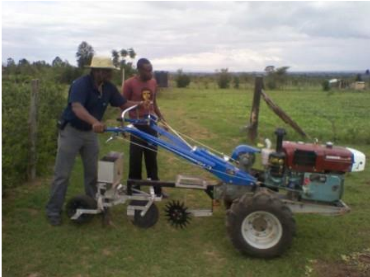
Dr. J. Mutua and Mr. I. Wahome setting the Morrison single row direct seeder ready for operation in Matanya Catholic church farm, Laikipia
