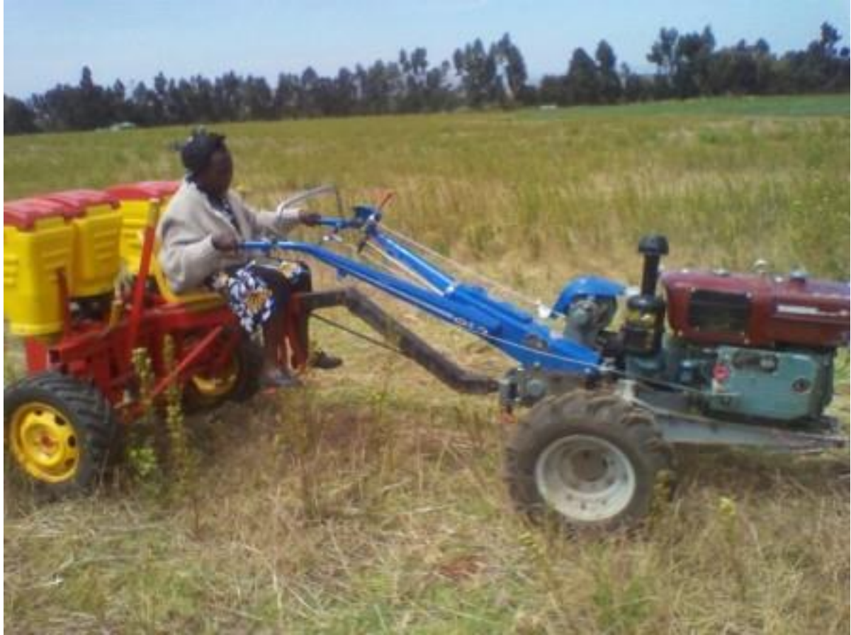
A trainee – the only lady in the training, planting with Fitarelli 2-row disc direct seeder in unploughed field
