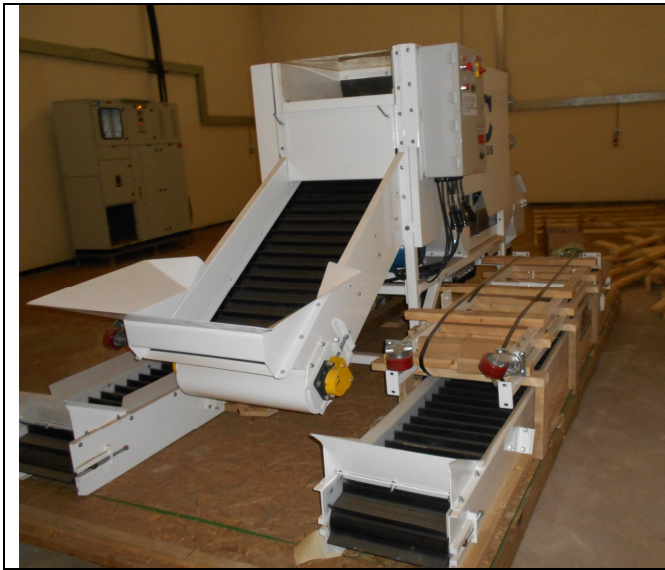
Seed shelling machine before installation
