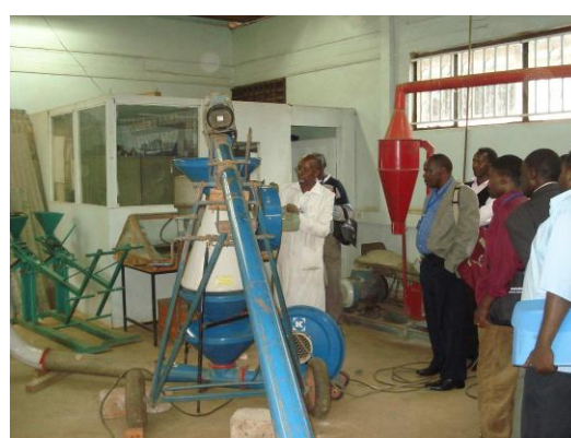
Mr Wanguhu from the seed laboratory at CAVS demonstrates how seed cleaning is done using machines
