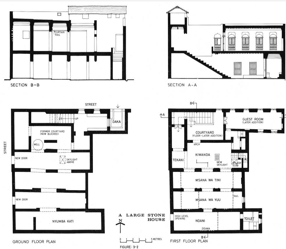
Fig24. Typical ground and first floor plans of a traditional stone house in the oldest section of Lamu town. (source: The Aga Khan award for architecture, conservation of Lamu, National Museum of Kenya)
