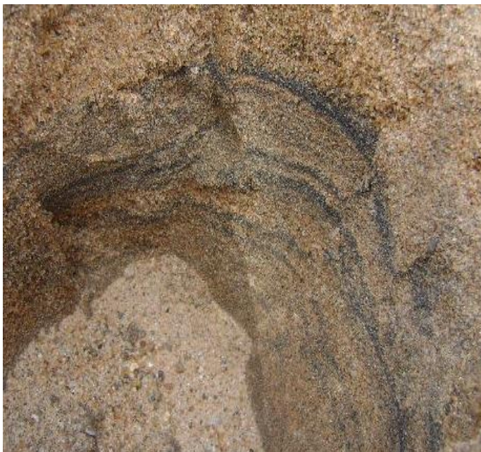
Figure 1-3: A cross section of a sampling site showing presence of heavy minerals
