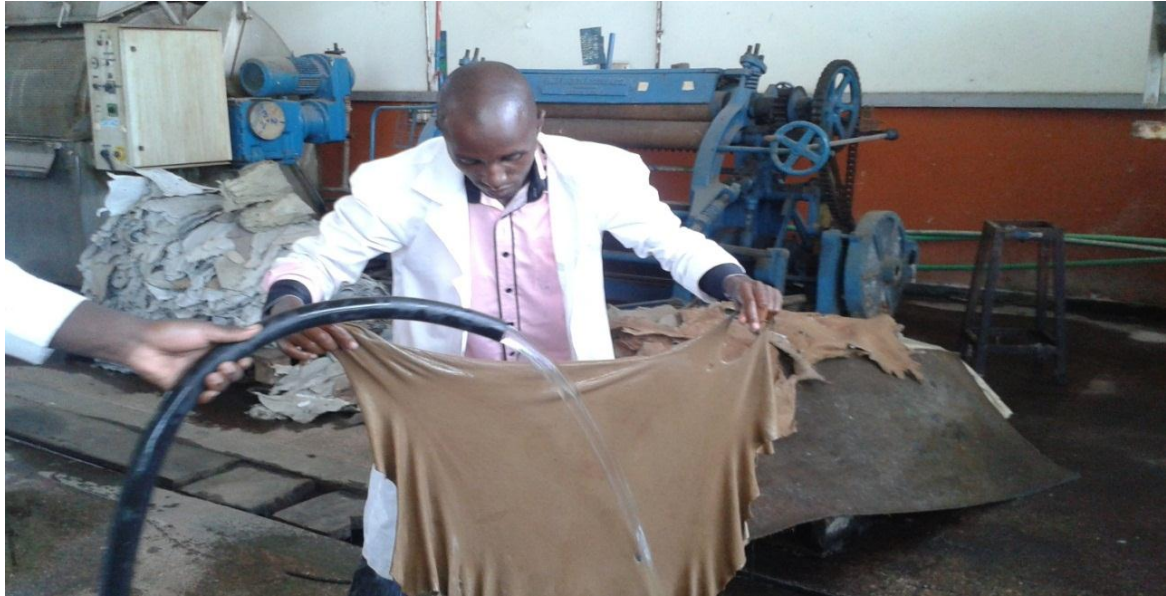
Plate 4.4: Fatliquored leather from Acacia nilotica before toggle drying
