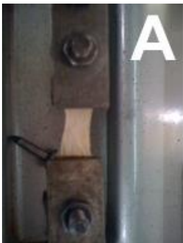
Figure 6:- Photographs showing a tissue sample being stretched to its ultimate tensile strength by the tensiometer.
