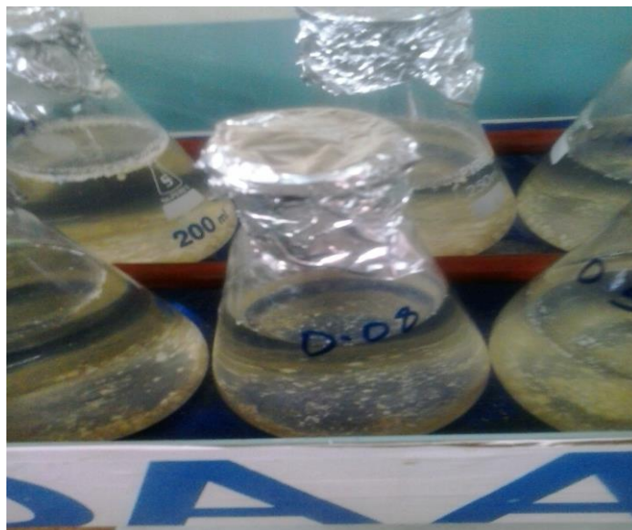
Figure 9. Water samples with various amount of M. oleifera seed powder on an orbital shaker.
