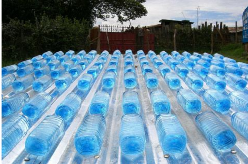
Figure 2. A sodis experiment set up
