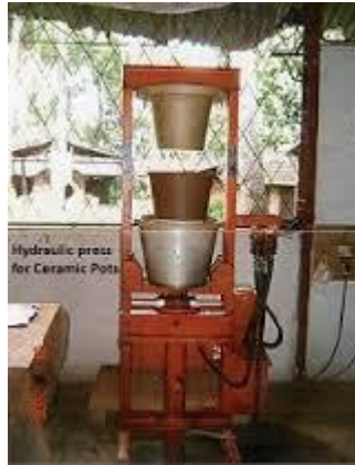
Figure 4. A hydraulic press for making frustum shaped filters
