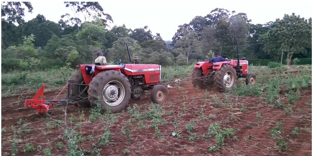
Plate 4.3: A trial run with the dynamometer anchored between the tractors
