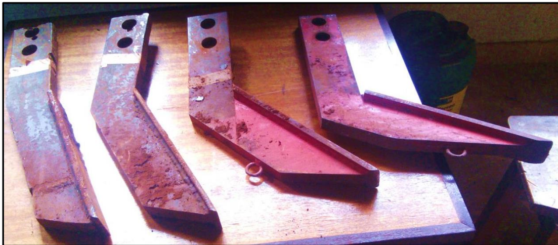
Figure 4.7: Ripper tines used (75°, 60°, 45° and 30° rake angles respectively)
