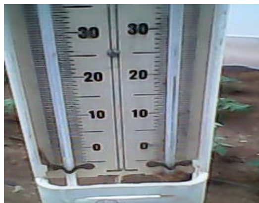
Figure 3.3: Measuring dry bulb and wet bulb temperatures within the greenhouse
