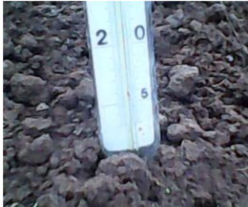
Figure 3.4: Measuring soil temperature at 10 cm depth inside the greenhouse
