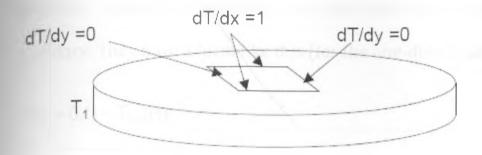
(b) 4 Dirichlet boundary condition on exterior boundary
