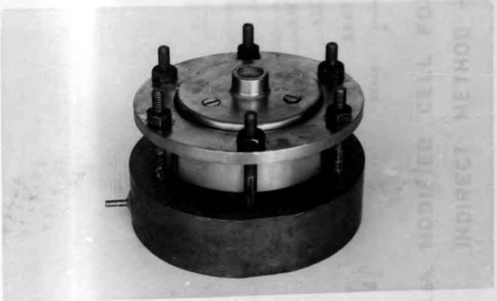
FIG.5.63. MODIFIED CELL FOR UNDISTURBED SOIL SAMPLE INDIRECT METHOD TEST SERIES A-2
