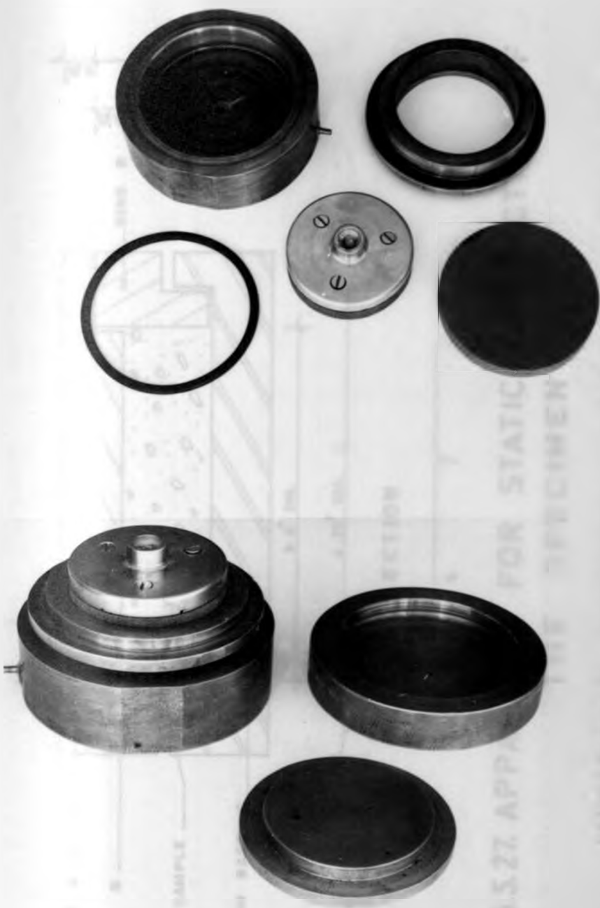
FIG.5.26. MODIFIED CELL FOR DISTURBED SOIL SAMPLE INDIRECT METHOD TEST SERIES A-1
