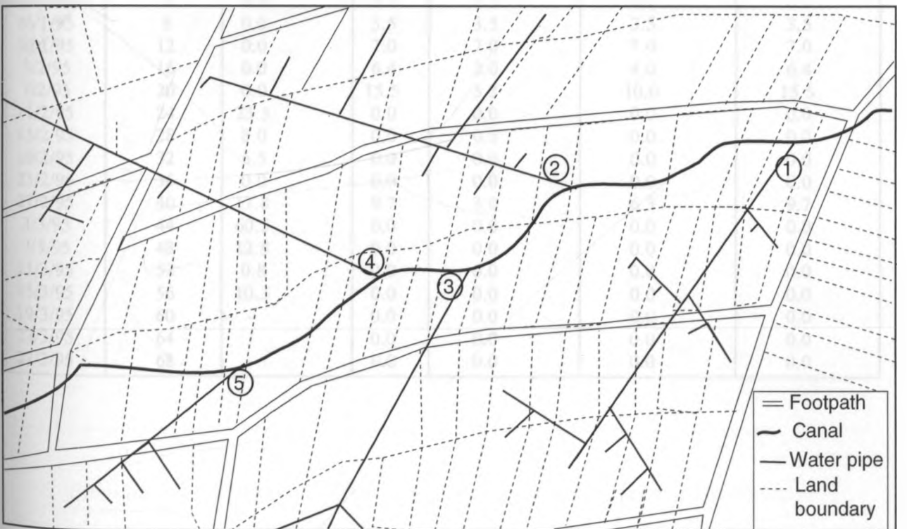
Figure 11: Alternative common point water delivery system for Aguthi Canal water users
