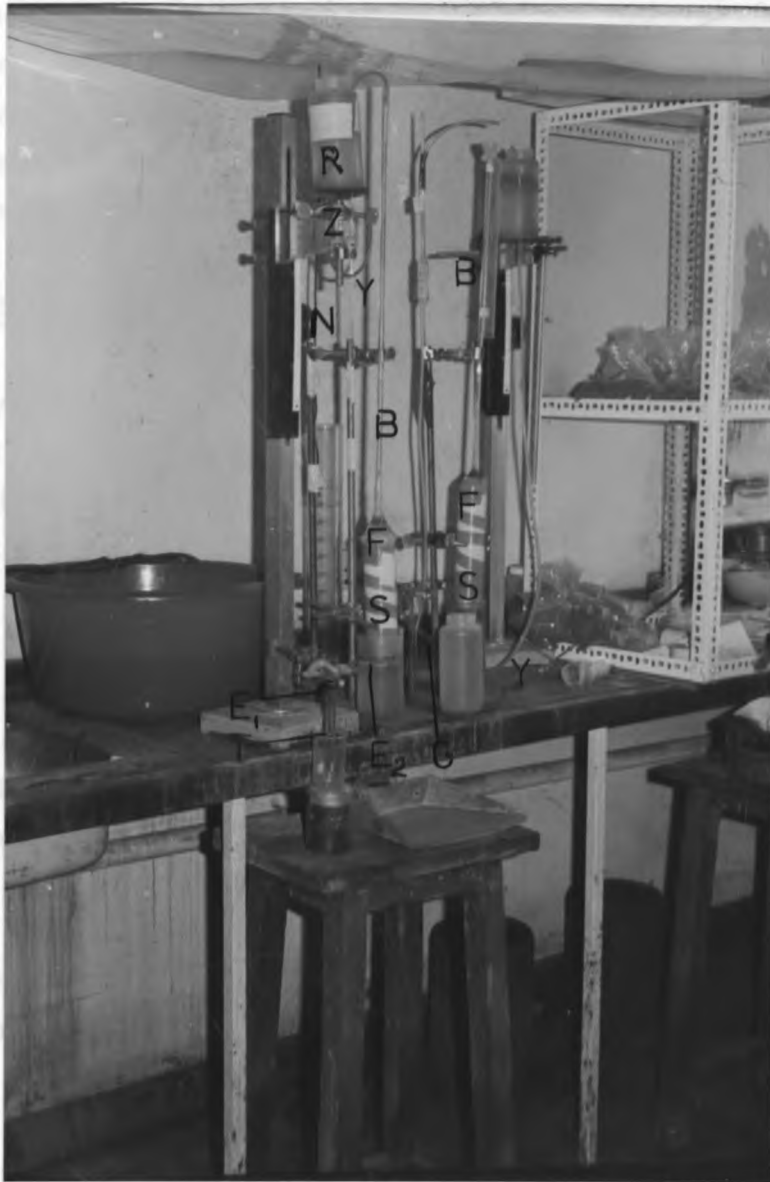
Plate 2-To show the set up the falling head apparatus.
