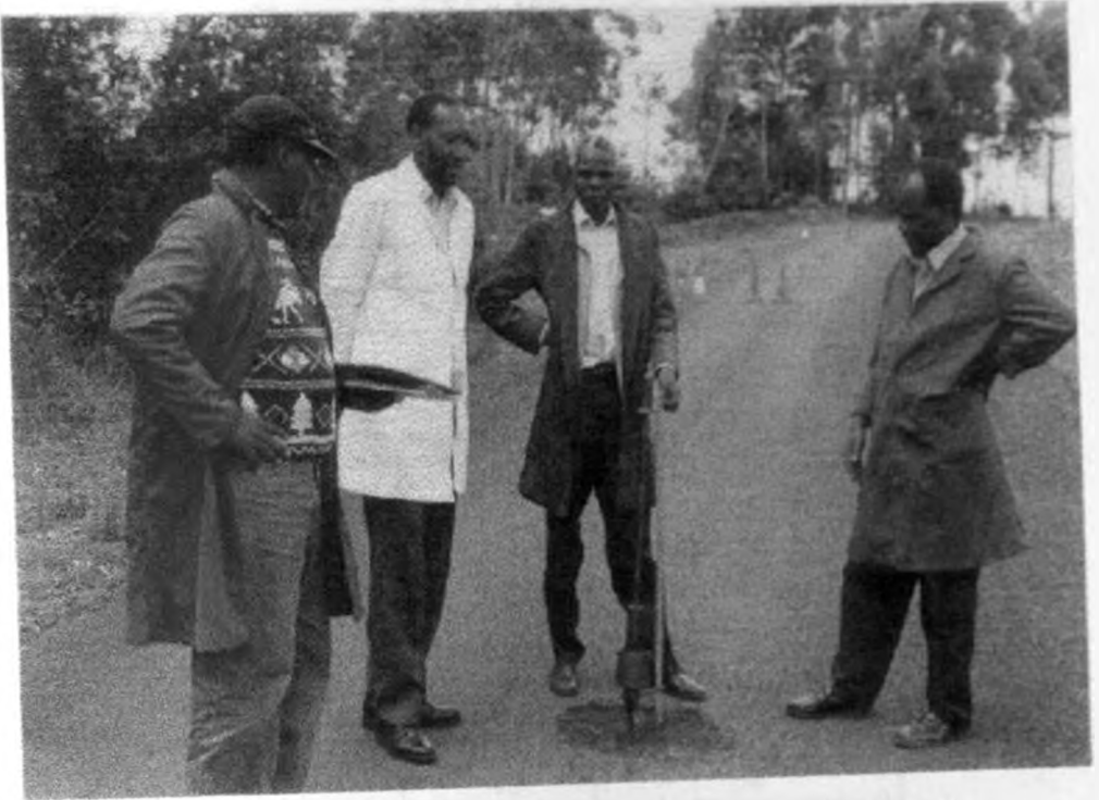
Plate A5.1 DCP at a pothole on ES9 after the 1997/98 El Nino rains
