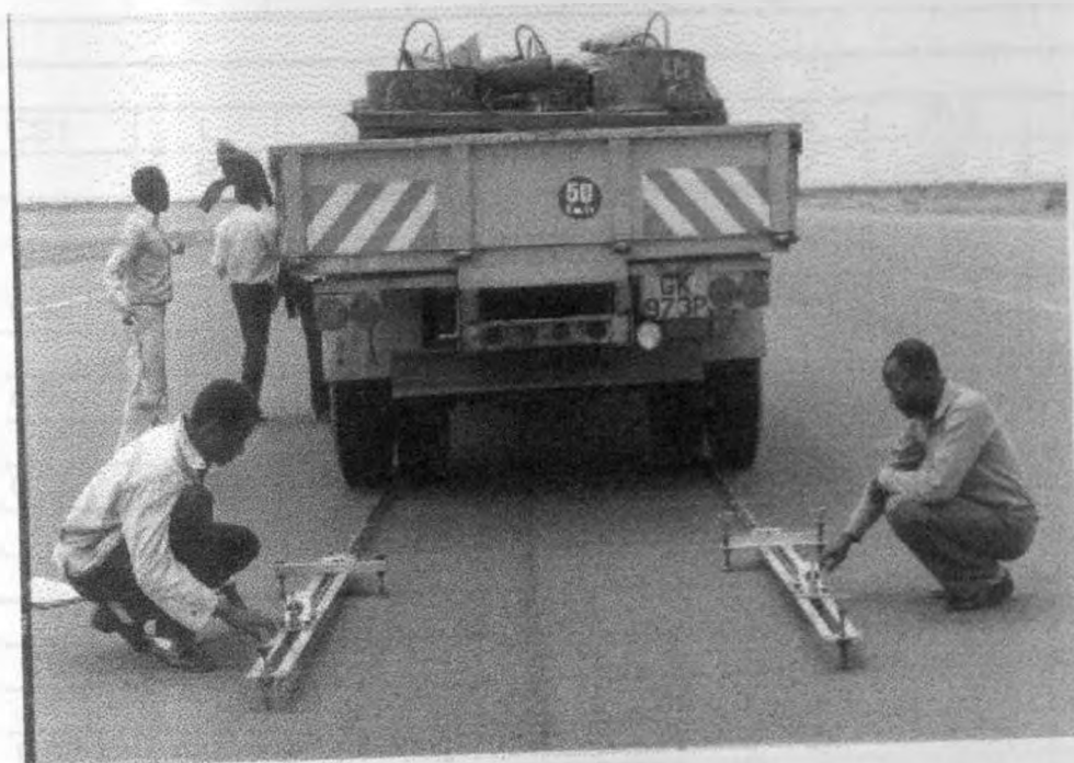
Plate A3.11 Benkleman beam and wheel arrangement during deflection measurements
