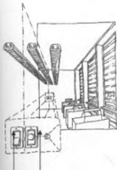
Automatic continuous dimming switch with photocell for the Daylighting Zone
