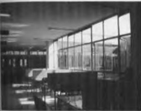
Reading Space next to Light Well abandoned due to direct sun falling on the reading desks, Source, ibid
