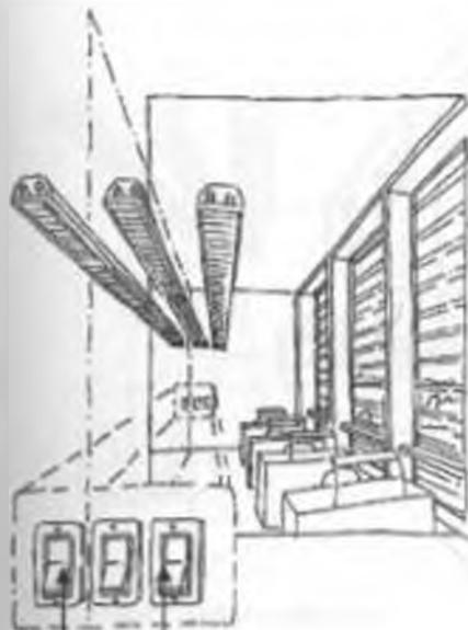
Two-level manual switch for the Daylighting Zone
