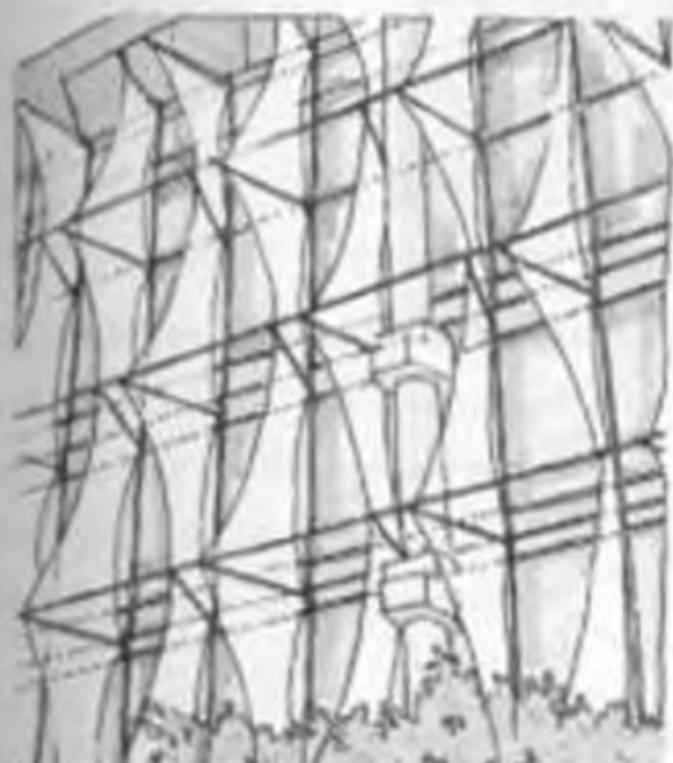
Vertical sunshade reduces glare from bright surroundings. The open design also allows view out and daylight penetration. This design should be augmented with internal shades for low perpendicular sun angles, source <http://www.libriadesign.org>
