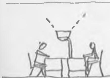
Localized lighting for visual task illumination is provided over the small area occupied by the task & immediate surrounding. There is less consumption of energy.
