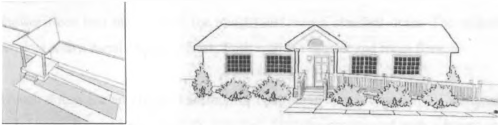
Figure 1: Ramps installed to upgrade an entrance
