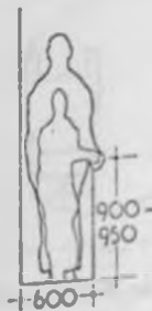
17.10 One person walking helped by a handrail. Height of handrail is a compromise between opposing criteria: the large man and the small elderly woman
