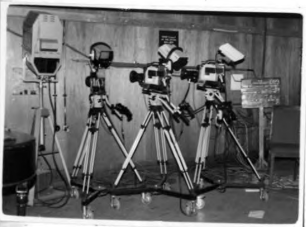
Plate 3.6 Television cameras used in the studio Note: - The smooth floor finish to aid the camera movement. - Also note the plywood panel absorbers
