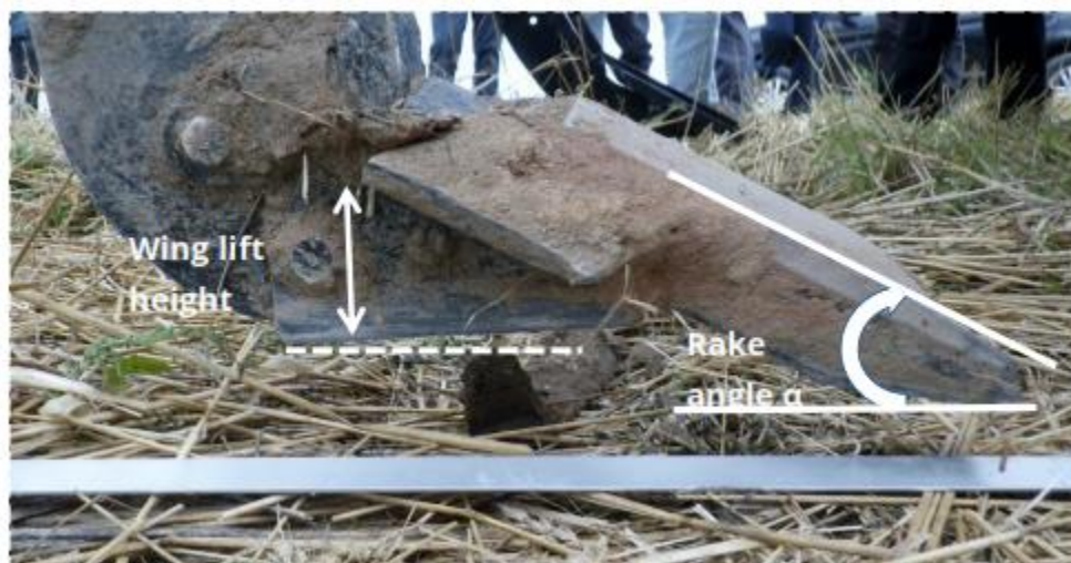
Figure 2.1: Wing lift height and Rake Angle (Source: A guide to successful Subsoiling - CETAB)
