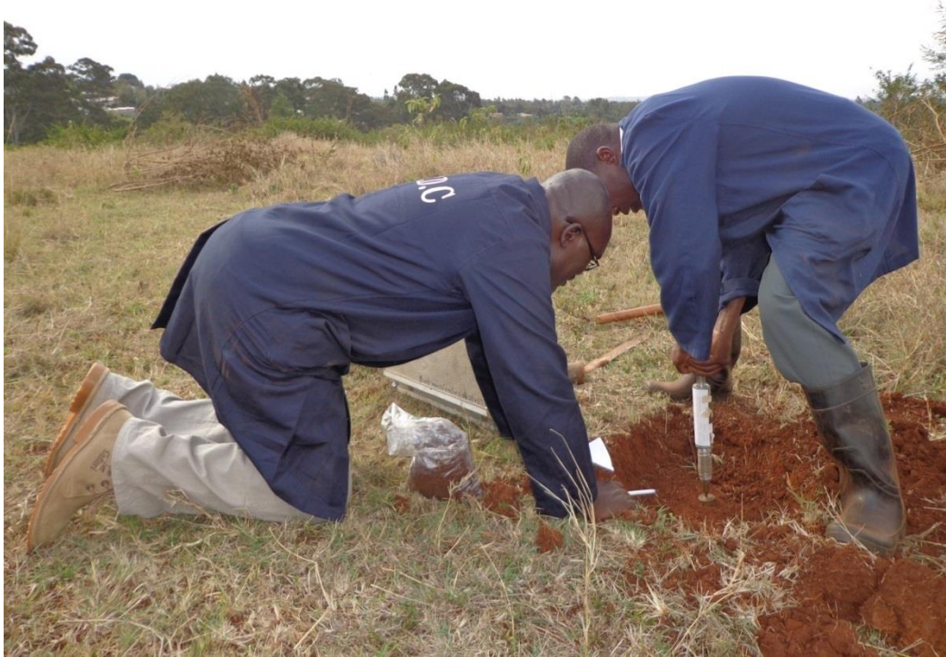
Plate 4.2: In-situ shear stress determination.
