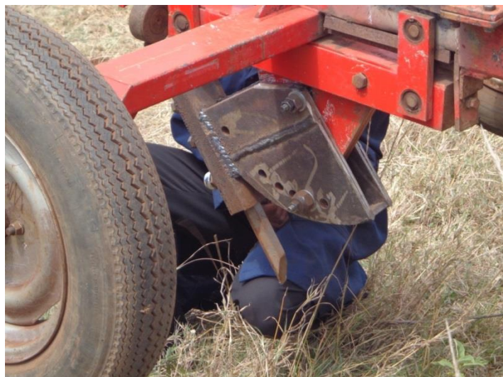
Plate 4.4: A sub-soiler mounted on the two wheeled frame for 60° rake angle
