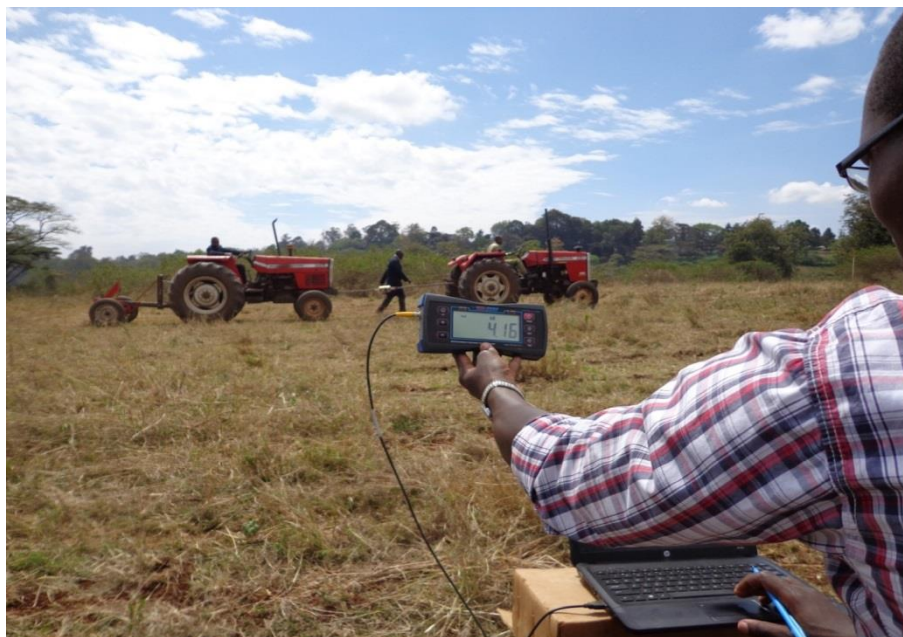
Plate 4.7: Monitoring and recording draft power on a digital datalogger.
