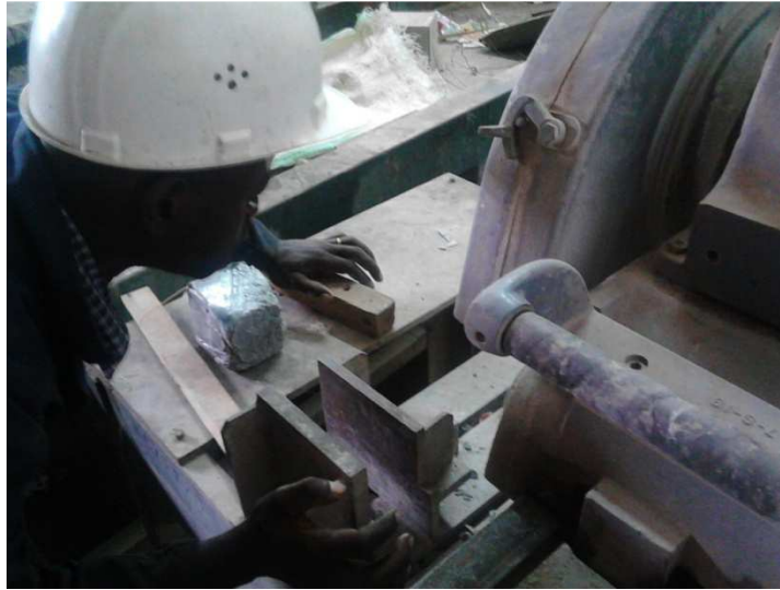
Figure 3.7: Cutting samples using rock saw for stereo microscopy
