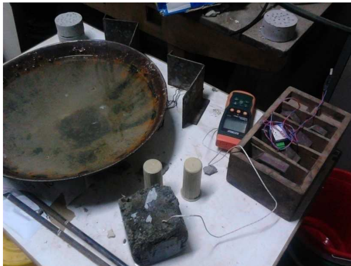
Figure 3.10: A complete set up with loggers in place for the samples to be cured under saturated conditions- 8th April 2015
