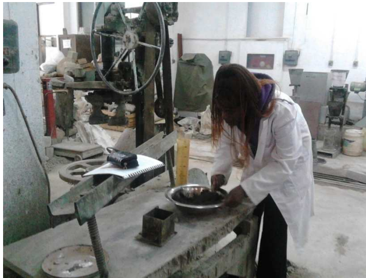
Figure 3.6: Mixing Ordinary Portland Cement paste in laboratories (University of Nairobi) -2nd April 2015
