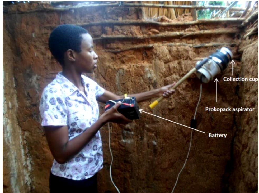
Figure 5: Image showing collection of indoor resting mosquitoes using a battery powered prokopack aspirator
