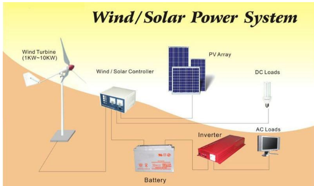
Figure 2-3: Solar-wind hybrid power system 1
