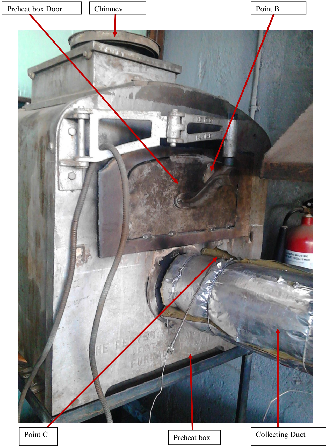
Figure 4. 3 Parts of preheating box and collecting duct
