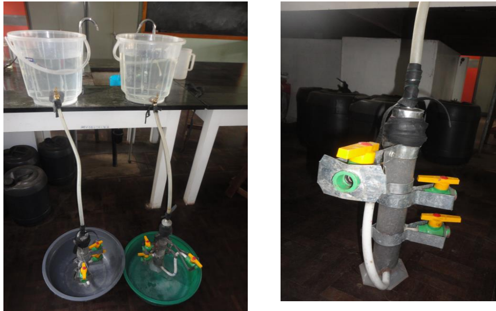
Plate 3.1: Experimental set up for Fixed Bed Adsorption Column Studies
