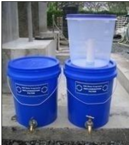
Figure 2. 2: Single and Combined Bone Char Filter (Eawag, 2006)
